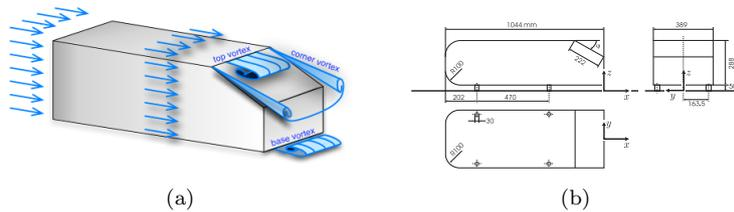
Figure 1: (a) Ahmed car body flow physics and (b) Ahmed car body dimensions
