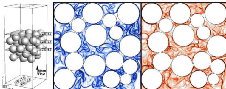
Figure : FTLE field computed from a turbulent flow through a packed bed
