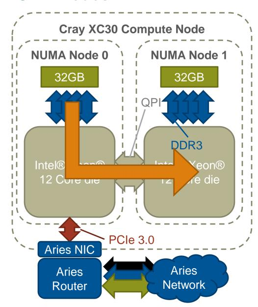
The design of the XC30 node means that CPUs accessing data stored on the other socket/die have to cross the QPI interprocessor bus
