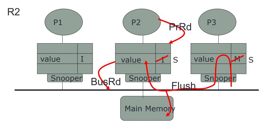
P2 wants to read the value. P3's cache has the most up-to-date copy and will provide it. P2's cache puts a BusRd on the bus. P3's cache snoops this and cancels the memory access because it will provide the data. P3's cache flushes the data to the bus.
