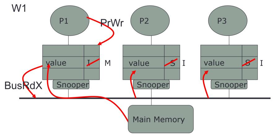
P1 wants to write to its cache. The cache places a BusRdX on the bus to gain exclusive access and the most up-to-date value. Main memory is not stale so it provides the data. The snoopers for P2 and P3 see the BusRdX and invalidate their copies in cache.
