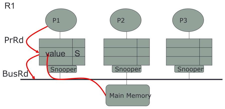
P1 wants to read the value. The cache does not have it and generates a BusRd for the data. Main memory controller provides the data. The data goes into the cache in the shared state.
