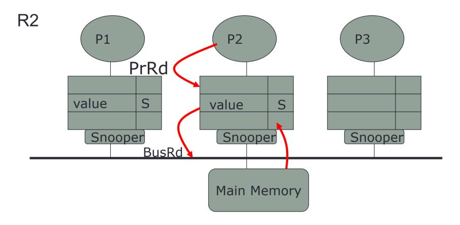
P2 wants to read the value. Its cache does not have the data, so it places a BusRd to notify other processors and ask for the data. The memory controller provides the data.
