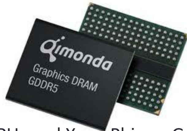
GPUs and Xeon Phi use Graphics DRAM
