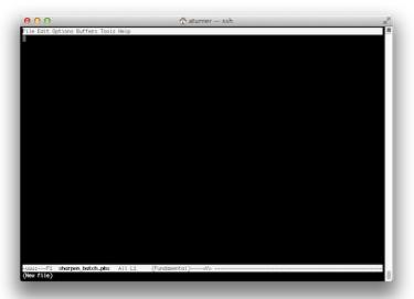
Typing will insert text as you would expect and backspace will delete text. You use special key sequences (involving the Ctrl and Alt buttons) to save files, exit Emacs and so on.
