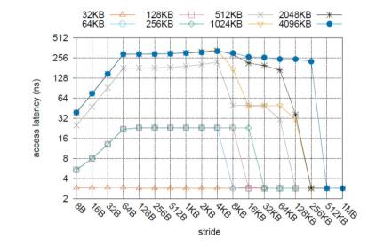
Fig. 4. Average memory latency when changing strides and datasets. The x-axis is logarithmic and it represents the pointer chasing stride.
