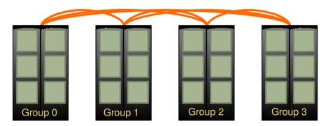
Example: An 4-group system is interconnected with 6 optical "bundles". The "bundles" can be configured between 20 and 80 cables wide
