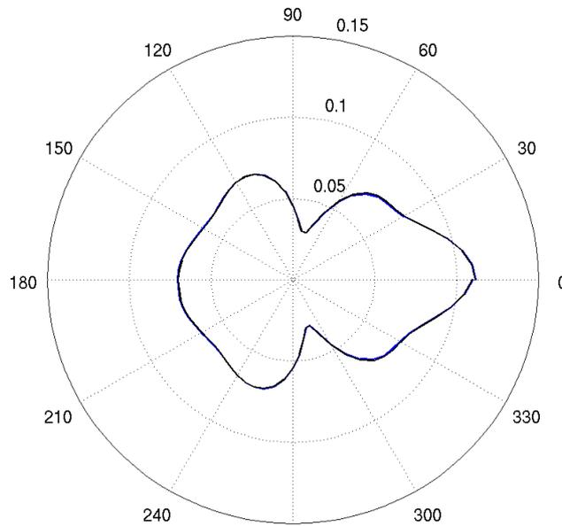
Figure 4: Directivity pattern for the scattered pressure from a rigid cylinder.
