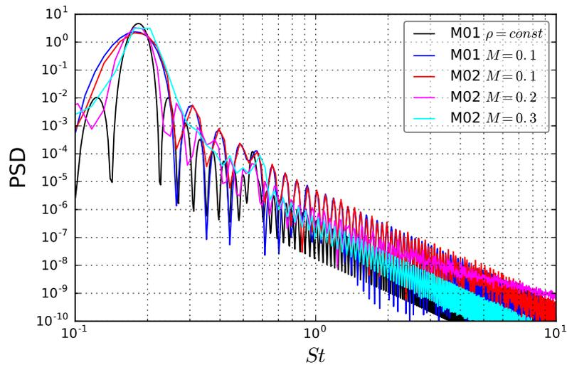
Figure 5: Comparison of the power spectral density of the lift coefficients  $C_L$  for different cases of the flow around a laminar cylinder at  $Re = 150$ .
