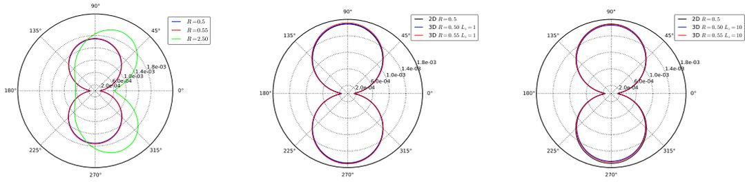
(a) Comparison between different integration surfaces. (b) Comparison between 2D and 3D meshes. The 3D one is obtained by extruding M01 with 5 layers to get a total span length of  $L_z = 1D$ . (c) Comparison between 2D and 3D meshes. The 3D one is obtained by extruding M01 with 51 layers to get a total span length of  $L_z = 10D$ .
