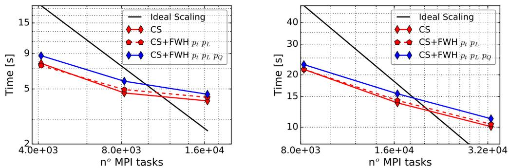
(a) Scalability test for the 3D mesh made of 38M cells. (b) Scalability test for the 3D mesh made of 150M cells.
