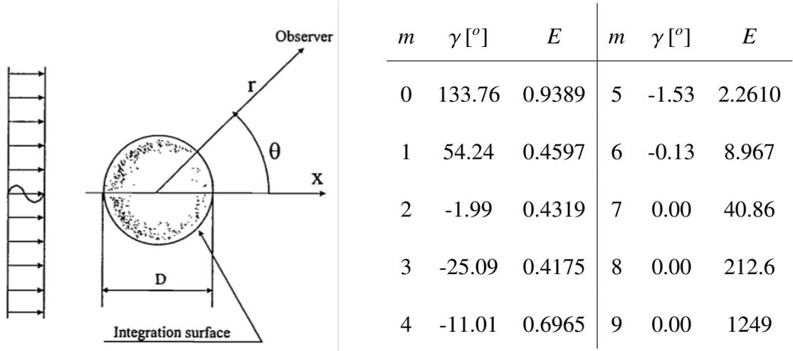
Figure 2: Sketch of the scattering of a plane wave by a rigid cylinder.
