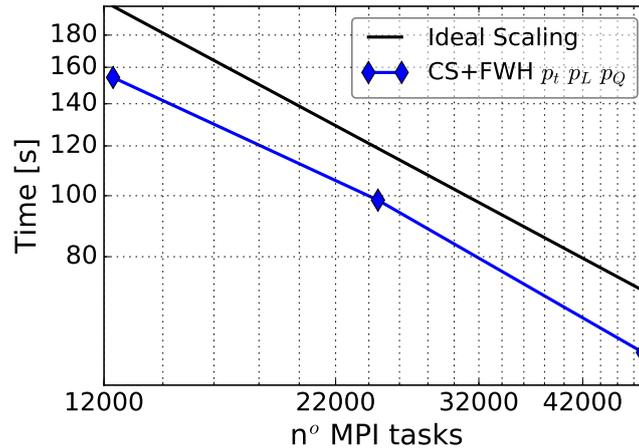
Figure 10: Scalability test for the 1.2 billion cell mesh on ARCHER.
