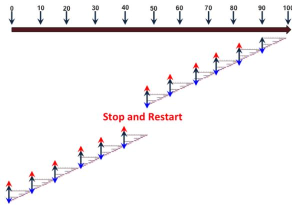
**Figure X.** For 100 time steps, the approach takes a state checkpoint every 10 forward timesteps. Then, in the reverse sweep, the state (and possibly adjoint) checkpoint is read, the adjoint is computed using binomial checkpointing, and the adjoint checkpoint is written.
